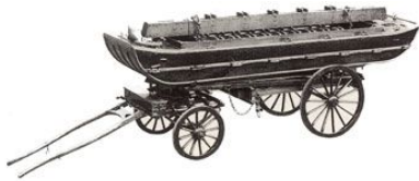
Blood Pontoon Mk. II designed by Lieutenant (later General Sir) Blood (1842-1940)
